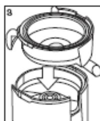
4. Put the filter in the juice collector. Ensure the filter is fitted securely onto the driving shaft. The blade should sit below the rim of the pulp container when in place.
