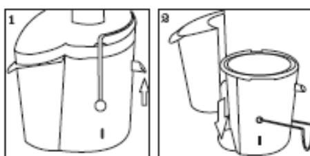
3. Place the juice collector into the appliance. Make sure the rim is flush with the motor unit.
