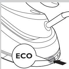
**1** To activate the ECO mode, press the ECO button. The light in the ECO button goes on.
