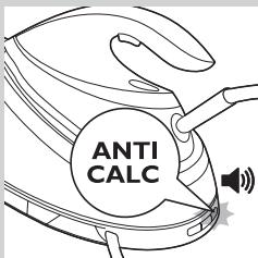
It is very important that you replace the ANTI-CALC cartridge when the ANTI-CALC cartridge replacement light starts flashing and the appliance starts beeping.
