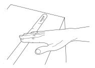
Due to the packaging of the sensor, it may have some wrinkles. After opening the package, prepare the sensor for use by smoothing out wrinkles on the sensor. Place the sensor on a hard surface and pat the wrinkles flat with your fingers. Getting just the largest wrinkles out is enough for correct operation.
