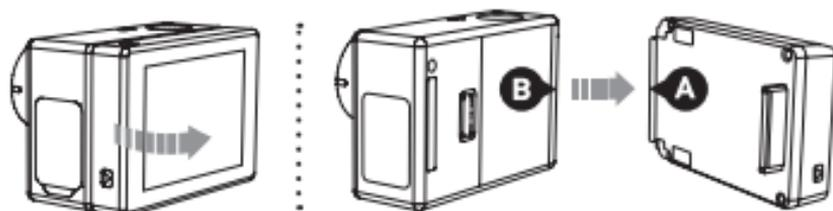
1. Pull back on left side of the LCD Touch BacPac marked with the arrow to disconnect from the HERO Port.
