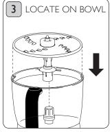
Place the spindle and shredding disc assembly onto the bowl drive of large processing bowl.
