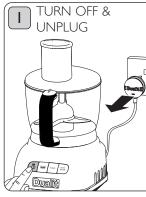
ALWAYS SWITCH OFF AND UNPLUG BEFORE ANY CLEANING. NEVER USE ABRASIVE CLEANERS ON ANY OF THE PARTS. TAKE EXTRA CARE WHEN WASHING BLADES.
