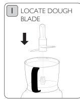
The dough blade can only be used with the large bowl. Place the dough blade directly onto the bowl drive in the large bowl.
