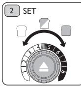
The toaster will only engage when To toast, set the desired browning level by means of the browning control (I is the lightest and 8 is the darkest setting).
