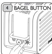
As soon as the bagel is lowered, immediately press the bagel button. The button will be illuminated blue and only the centre element will heat up.
