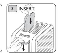
press the toasting lever down until it engages. The browning control will be illuminated blue for the duration of the toasting.
