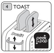
Place the bread into the slots and At any time during the toasting cycle you can lift the toasting lever and check the progress of the bread. When toasted the toast will pop up automatically.
