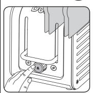
To immediately stop toasting, simply press the cancel button on the end of the browning control knob. Unplug after use.
