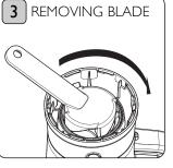
To remove the blades use the tool provided. Insert and rotate the blades **CLOCKWISE TO** LOOSEN. Continue to unscrew and lift to remove.
