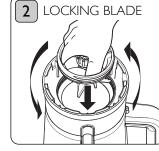
Align the blade assembly to base of the jar. Using your fingers, **ROTATE** ANTI-CLOCKWISE TO **TIGHTEN** then use the tool to lock in to place.
