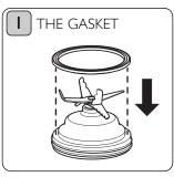
Ensure the gasket is seated on the collar of the blade correctly before inserting into the jar. It can be placed on either way round.
