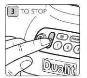
To stop blending, press the stop button at any time, this will be illuminated red. Always turn main power off & unplug after each use.
