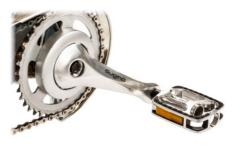
Lubricate the moving parts and keep the tension on the chain just so that if you press in the middle, it gives away 1 cm.
