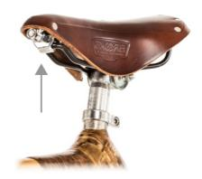
For the right maintenance of your saddle, you should adjust the bolt fitted under the saddle every two months. This can be done with your BROOKS saddle tension spanner provided in the box. For the exact details check your BROOKS maintenance instructions. Also tighten the grips with the allen key if it's too loose.
